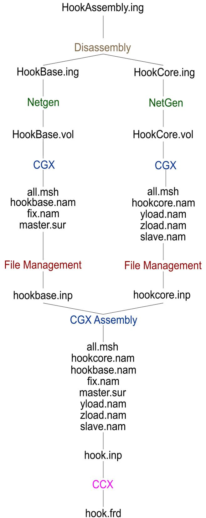
9. Repeating this for the next body will end up in just two different .inp files that will be use for the construction of the model, notice that by this point the two bodies are not assembled there are just defined with is sets independently.
